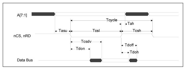
Figure 6.2 PIO Read Cycle Timing
