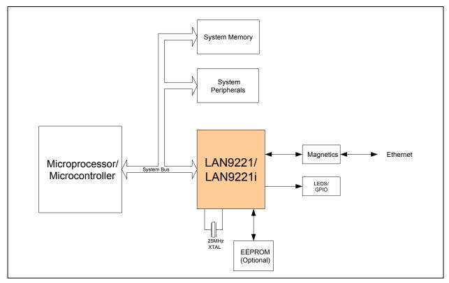
Figure 1.1 System Block Diagram
