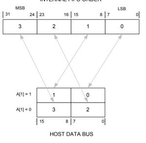
Figure 3.3 FIFO Access Byte Ordering
