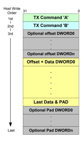
Figure 3.14 TX Buffer Format
