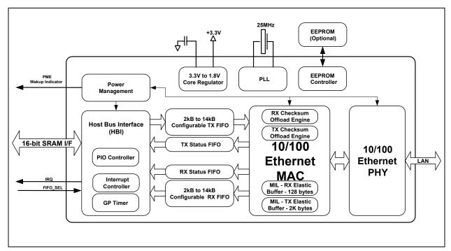
Figure 1.2 Internal Block Diagram
