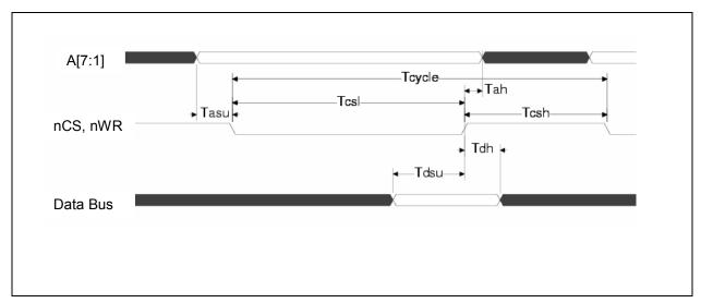
Figure 6.6 PIO Write Cycle Timing
