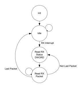
Figure 3.18 Host Receive Routine Using Interrupts
