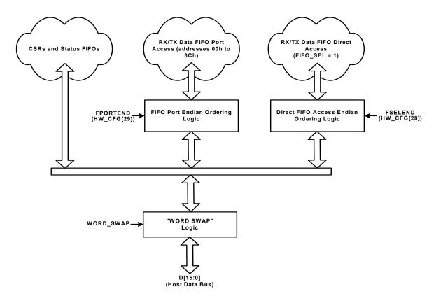
Figure 3.2 LAN9221/LAN9221i Host Data Path Diagram
