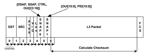
Figure 3.8 Ethernet Frame with VLAN Tag and SNAP Header
