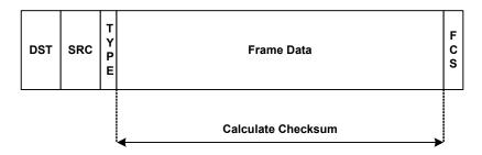
Figure 3.4 RXCOE Checksum Calculation
