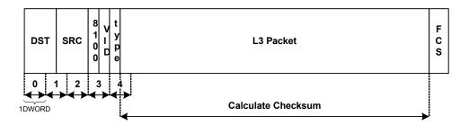
Figure 3.6 Ethernet Frame with VLAN Tag
