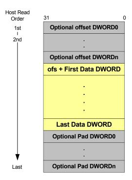
Figure 3.20 RX Packet Format
