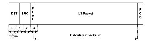
Figure 3.5 Type II Ethernet Frame
