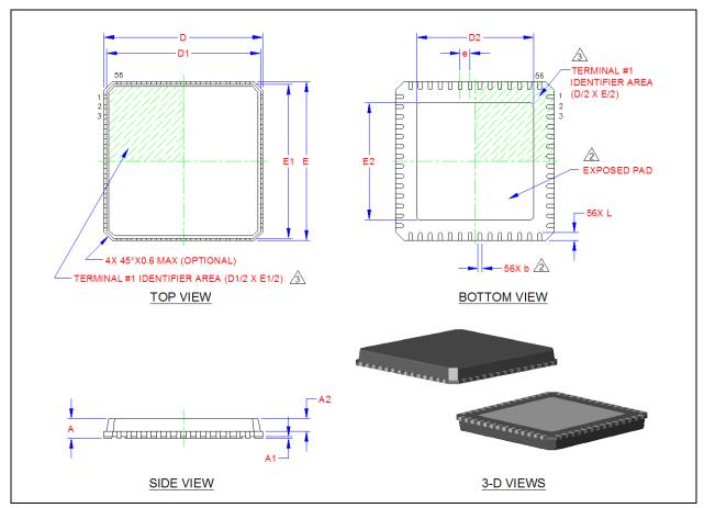
Figure 8.1 56 Pin QFN Package Definition
