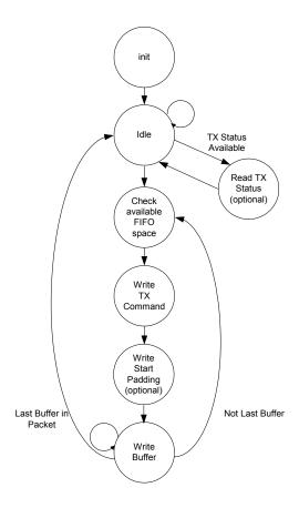
Figure 3.13 Simplified Host TX Flow Diagram
