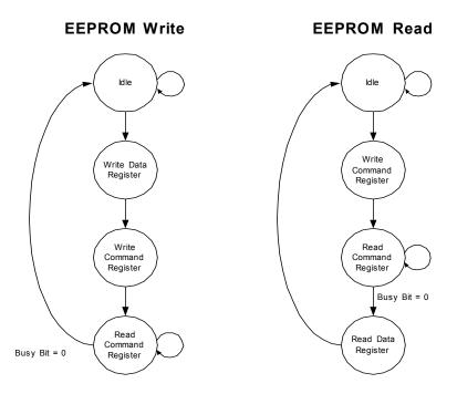
Figure 3.4 EEPROM Access Flow Diagram
