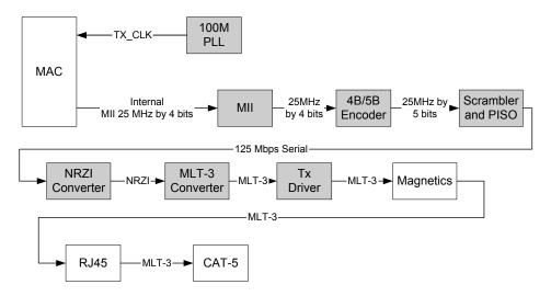
Figure 4.1 100Base-TX Data Path
