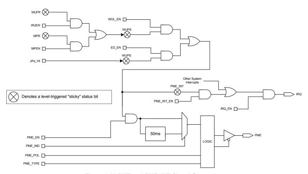
Figure 3.12 PME and PME\_INT Signal Generation
