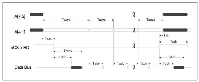
Figure 6.3 PIO Burst Read Cycle Timing
