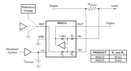
NOTE: 1-MW paths from shunt inputs to reference and INA21x outputs.
