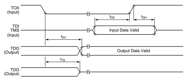
Figure 10-16 Test Access Port Timing Diagram
