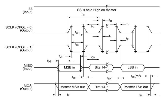
Figure 10-7 SPI Master Timing (CPHA = 0)
