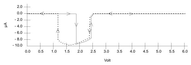
Figure 10-1  $I_{IN}/I_{OZ}$  vs. Voltage (Typical)
