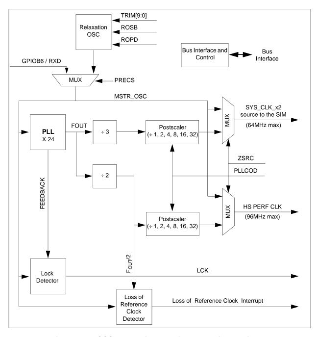
Figure 3-2 OCCS Block Diagram with Relaxation Oscillator
