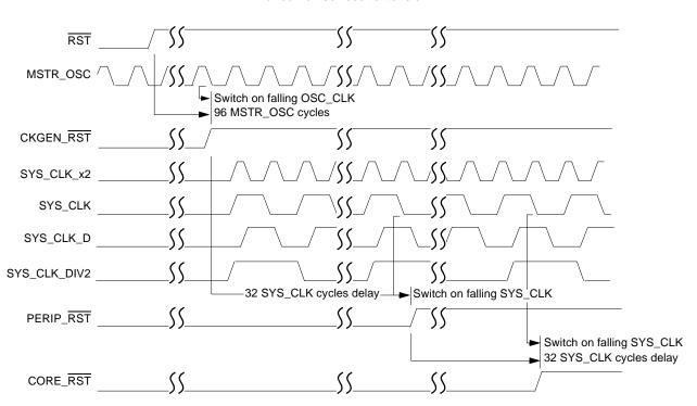
Maximum Delay = 64 MSTR\_OSC cycles for POR reset extension and 32 MSTR\_OSC cycles for combined reset extension
