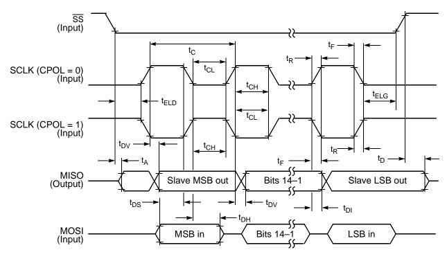
Figure 10-10 SPI Slave Timing (CPHA = 1)
