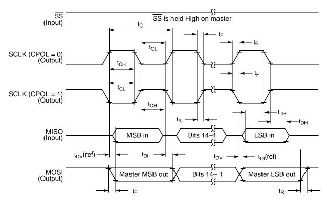
Figure 10-8 SPI Master Timing (CPHA = 1)
