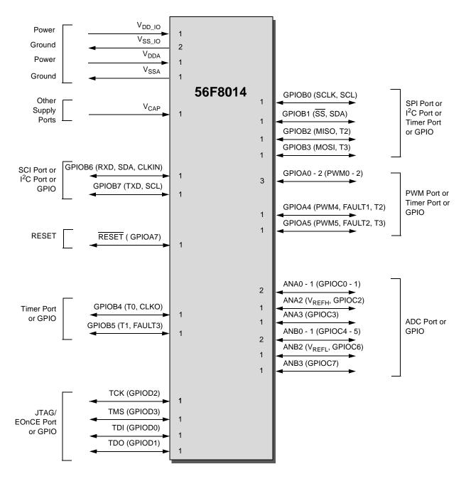
Figure 2-1 56F8014 Signals Identified by Functional Group (32-Pin LQFP)
