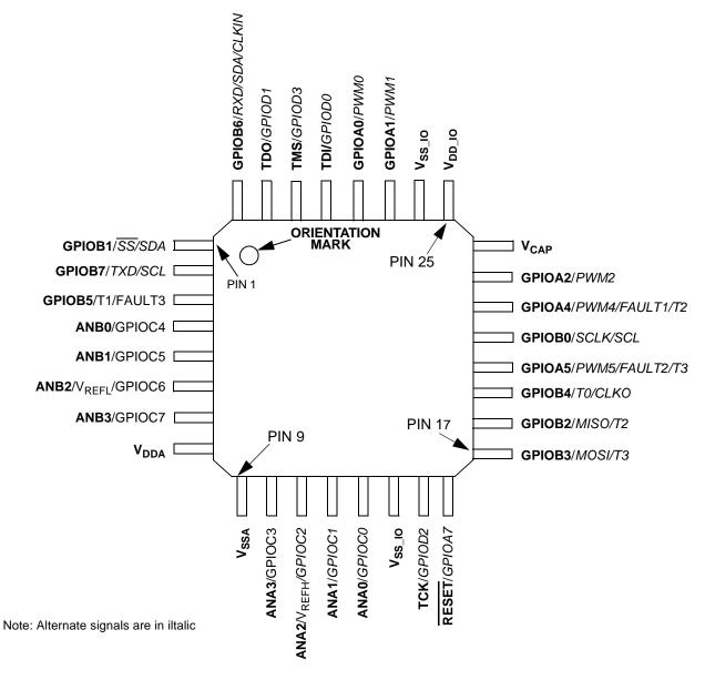
Figure 11-1 Top View, 56F8014 32-Pin LQFP Package
