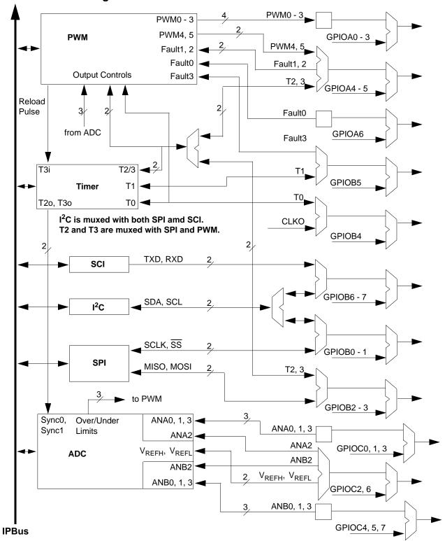
Figure 1-3 56F8014 Peripheral I/O Pin-Out
