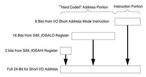
Figure 6-12 I/O Short Address Determination
