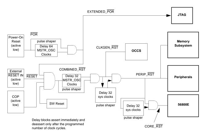
Figure 6-15 Sources of RESET Functional Diagram (Test modes not included)
