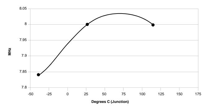
Figure 10-5 Relaxation Oscillator Temperature Variation (Typical)
