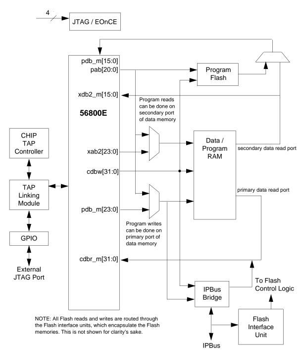
Figure 1-1 System Bus Interfaces
