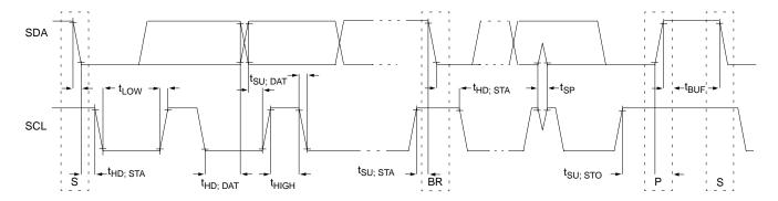
Figure 10-14 Timing Definition for Fast and Standard Mode Devices on the I<sup>2</sup>C Bus
