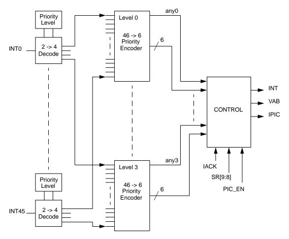
Figure 5-1 Interrupt Controller Block Diagram
