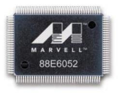
The shared memory-based switch fabric uses Marvell's latest switch architecture that provides non-blocking switching performance in all traffic environments. Back-pressure and pause frame-based flow control schemes are supported to ensure zero packet loss under traffic congestion. The look-up engine allows for up to 4,096 active nodes to be connected with the switch.
