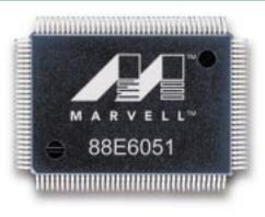
Advanced voice/video/data networking capability is supported by the Marvell 88E6051/88E6052 devices' Quality of Service (QoS) wire-speed non-blocking switch fabric with four priority queues per switch port, which can segment packet streams into network management, voice, video, and data packets. In addition, port-based VLAN and packet priority tagging features prioritize packet transfers for each switch port's egress queue, minimizing latency and enhancing QoS.
