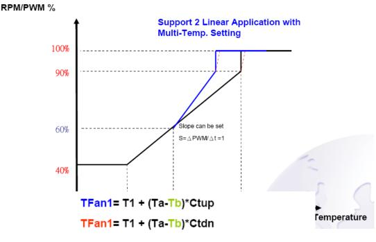
1. **Ctup**, **Ctdn** Can be Programmed to 1, <sup>1</sup>/<sub>2</sub>, <sup>1</sup>/<sub>4</sub>, 0 2. **Ta** Can be Selected to the Same Temp. Source (Ex:T1)
