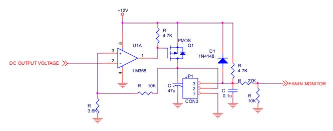
Figure 5 DAC fan control application circuit
