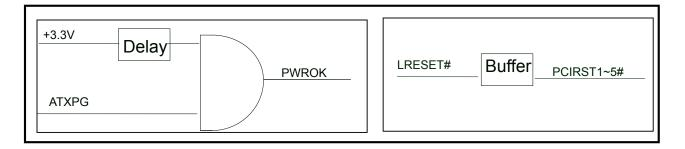
So far as the PWROK issue is as the figure above. PWROK is delayed 400ms (default) as VCC arrives 2.8V, and the delay timing can be programmed by register. An additional delay could be added to PWROK (0ms, 100ms, 200ms and 400ms). If RSTCION# and PCIRST4#/PCIRST5# are enabled, RSTCON# could be programmed to be asserted via PWROK or PCIRST4#/PCIRST5#.
