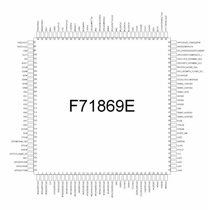
Figure1. F71869E pin configuration (14 \*14)
