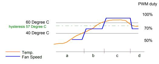
Figure 9 Stage mode fan control illustration-2
