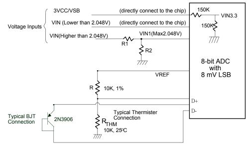
Figure 2. Hardware monitor configuration
