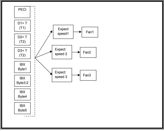
Figure 7 Relative temperature fan control
