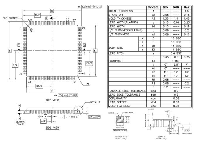
Figure 19 128 Pin LQFP Package Diagram
