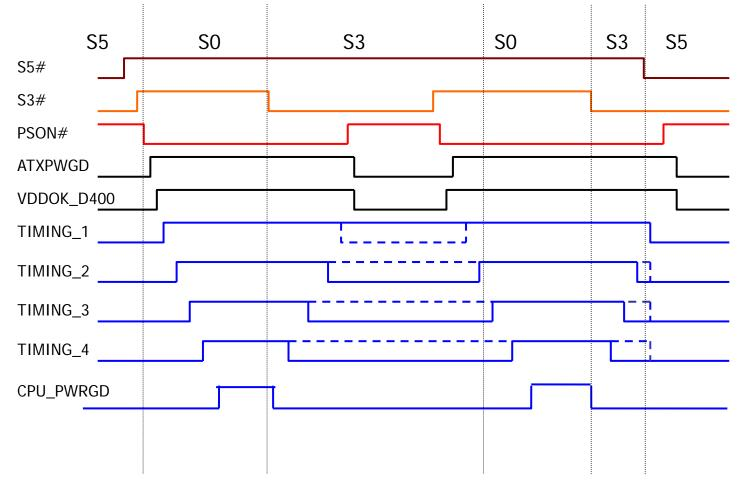
Figure 14 Timing on/off sequence
