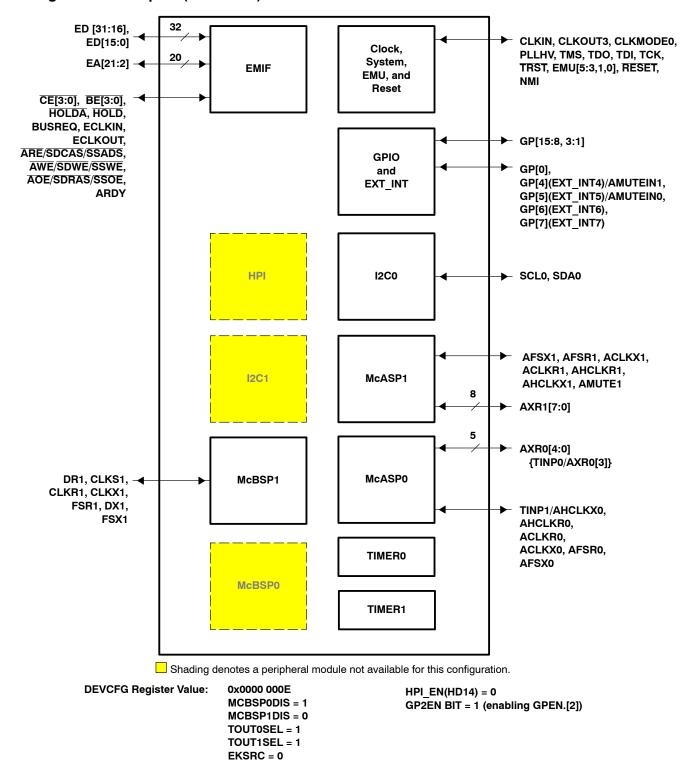
Figure 7. Configuration Example B (1 I2C + 1 McBSP + 2 McASP + GPIO)
