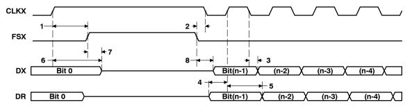
Figure 61. McBSP Timing as SPI Master or Slave: CLKSTP = 10b, CLKXP = 1
