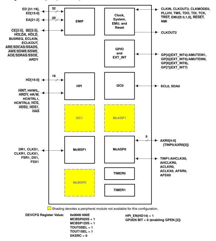
Figure 11. Configuration Example F (1 McBSP + HPI + 1 McASP)
