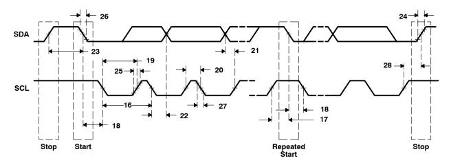
Figure 52. I<sup>2</sup>C Transmit Timings
