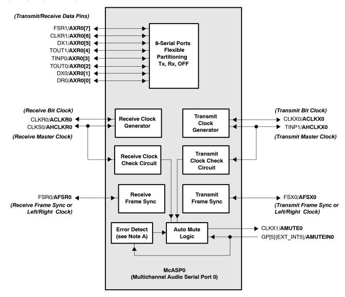
NOTES: A. The McASPs' Error Detect function detects underruns, overruns, early/late frame syncs, DMA errors, and external mute input.
