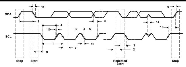
Figure 51. I<sup>2</sup>C Receive Timings
