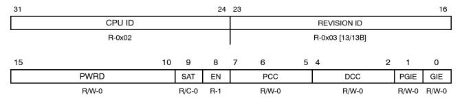
Legend: R = Readable by the MVC instruction, R/W = Readable/Writeable by the MVC instruction; W = Read/write; -n = value after reset, -x = undefined value after reset, C = Clearable by the MVC instruction
