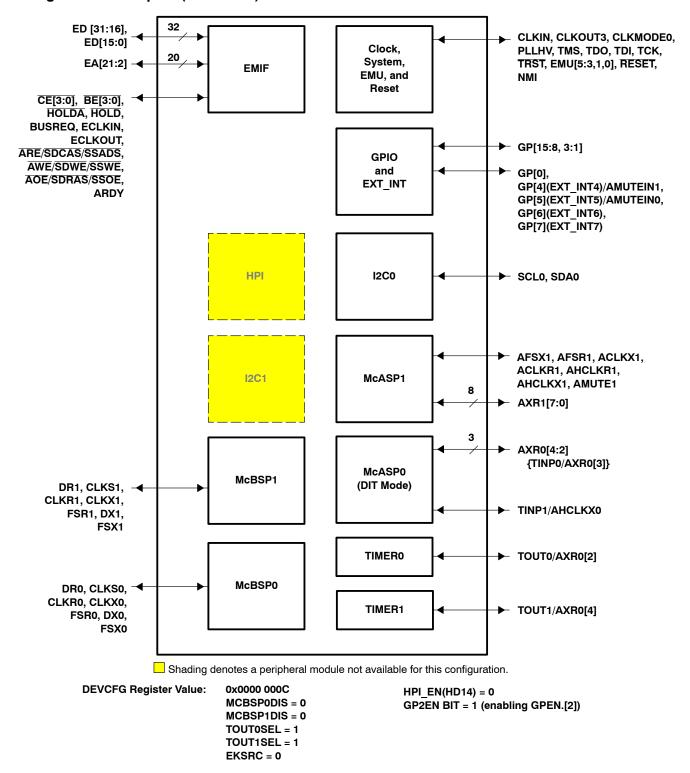
Figure 9. Configuration Example D [1 I2C + 2 McBSP + 1 McASP + 1 McASP (DIT) + GPIO + Timers]
