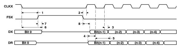
Figure 59. McBSP Timing as SPI Master or Slave: CLKSTP = 10b, CLKXP = 0
