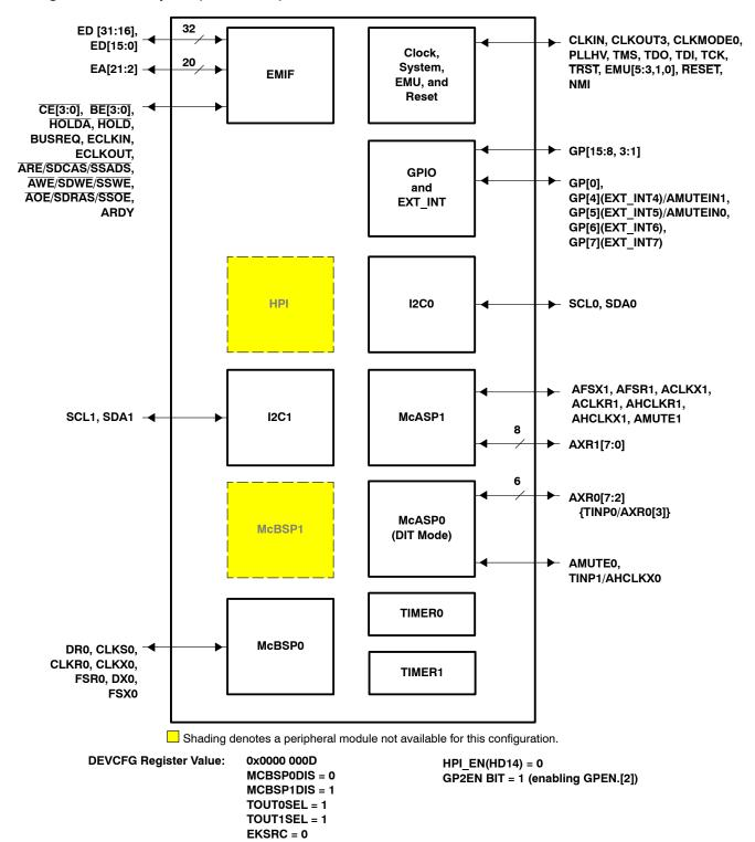
Figure 8. Configuration Example C [2 I2C + 1 McBSP + 1 McASP + 1 McASP (DIT) + GPIO]
