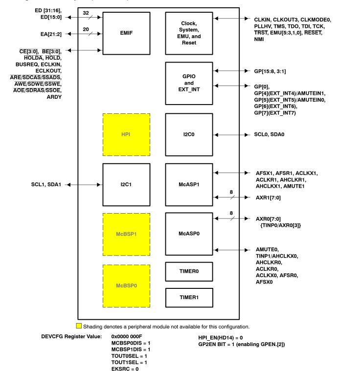
Figure 6. Configuration Example A (2 I2C + 2 McASP + GPIO)
