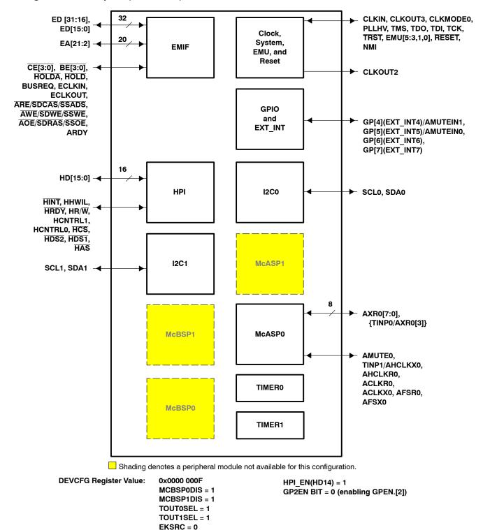
Figure 10. Configuration Example E (1 I2C + HPI + 1 McASP)
