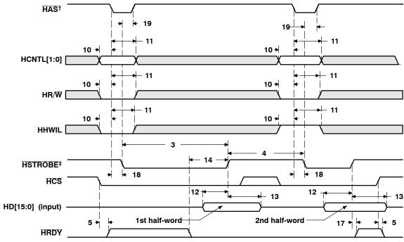
$<sup>^\</sup>dagger$  For correct operation, strobe the  $\overline{\text{HAS}}$  signal only once per  $\overline{\text{HSTROBE}}$  active cycle.
