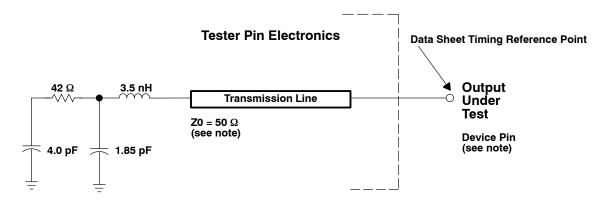
NOTE: The data sheet provides timing at the device pin. For output timing analysis, the tester pin electronics and its transmission line effects must be taken into account. A transmission line with a delay of 2 ns or longer can be used to produce the desired transmission line effect. The transmission line is intended as a load only. It is not necessary to add or subtract the transmission line delay (2 ns or longer) from the data sheet timings.
