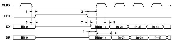
Figure 60. McBSP Timing as SPI Master or Slave: CLKSTP = 11b, CLKXP = 0
