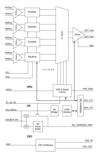
The PS421 supports either fixed cable equalization with default setting of 10-dB at 1.65Gbps and 12-dB at 2.25Gbps receiver equalization, or programmable equalization from 0 to 14-dB/16-dB (1.65Gbps/2.25Gbps) by pin selection or I2C control registers.
