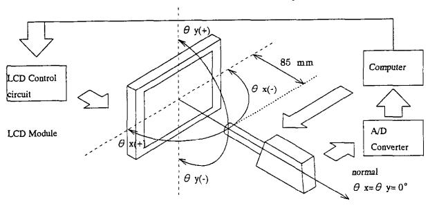
(Measuring spot size :  $\phi$  10 mm, Measuring Field : 2 °)
