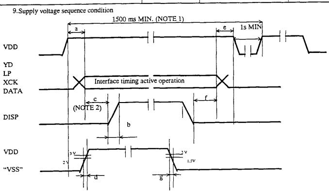
Fig.12 Supply voltage sequence condition
