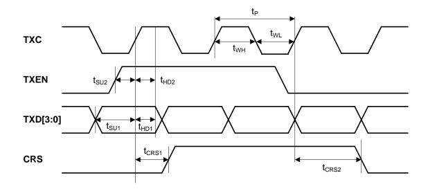
Figure 12. MII Transmit Timing (10Base-T)
