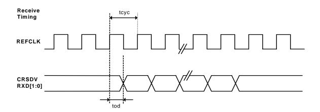
Figure 17. RMII Timing - Data Input to RMII
