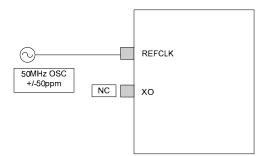
Figure 7. 50MHz Oscillator Reference Clock for RMII Mode
