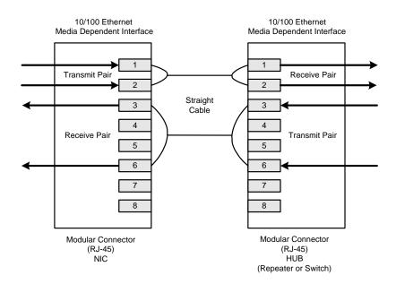
Figure 4. Typical Straight Cable Connection
