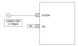
Figure 8. 125MHz Oscillator Reference Clock for SMII Mode
