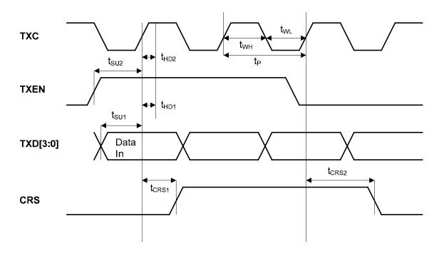
Figure 14. MII Transmit Timing (100Base-TX)
