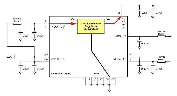
Figure 9. KSZ8041TL/FTL Power and Ground Connections
