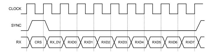
Figure 3. SMII Receive Data/Control Segment
