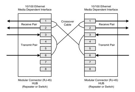
Figure 5. Typical Crossover Cable Connection
