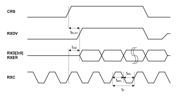
Figure 15. MII Receive Timing (100Base-TX)
