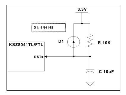
Figure 21. Recommended Reset Circuit
