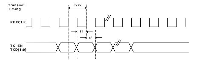
Figure 16. RMII Timing - Data Received from RMII
