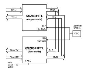
Figure 10. KSZ8041FTL / KSZ8041TL Back-to-Back Media Converter
