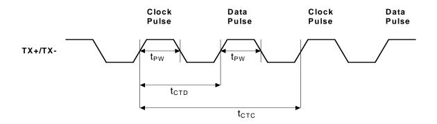
Figure 18. Auto-Negotiation Fast Link Pulse (FLP) Timing
