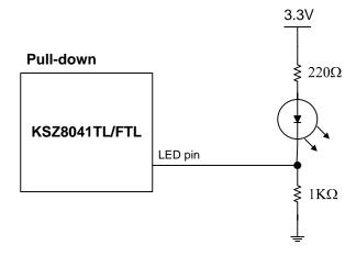
Figure 23. Reference Circuits for LED Strapping Pins
