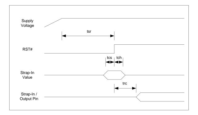
Figure 20. Reset Timing
