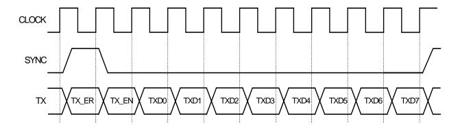
Figure 2. SMII Transmit Data/Control Segment
