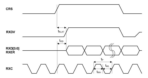
Figure 13. MII Receive Timing (10Base-T)
