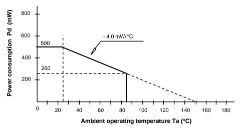
Remark: The main component of power consumption by this IC is the power consumed by the output transistors on channels 1 to 4.
