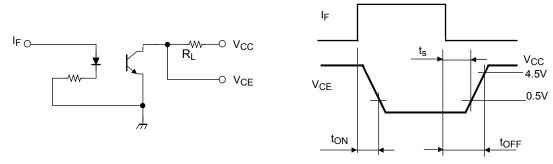
(Note 5): Switching time test circuit
