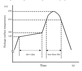
This profile is based on the device's maximum heat resistance guaranteed value.
