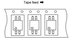
**Figure 1 Device Orientation**
