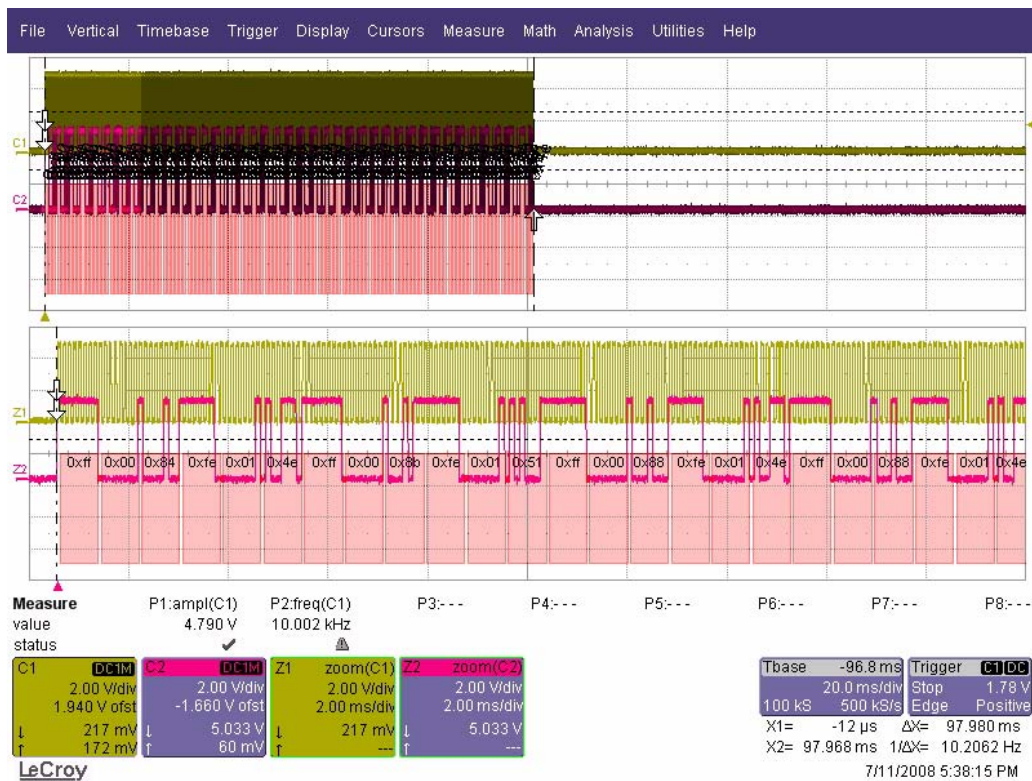
Figure 3-7. RF Telegram Received and Decoded
