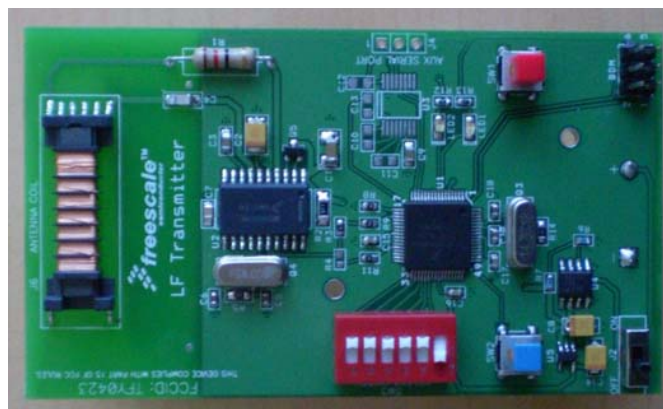
Figure 1-4. LF 125 kHz Emitter
