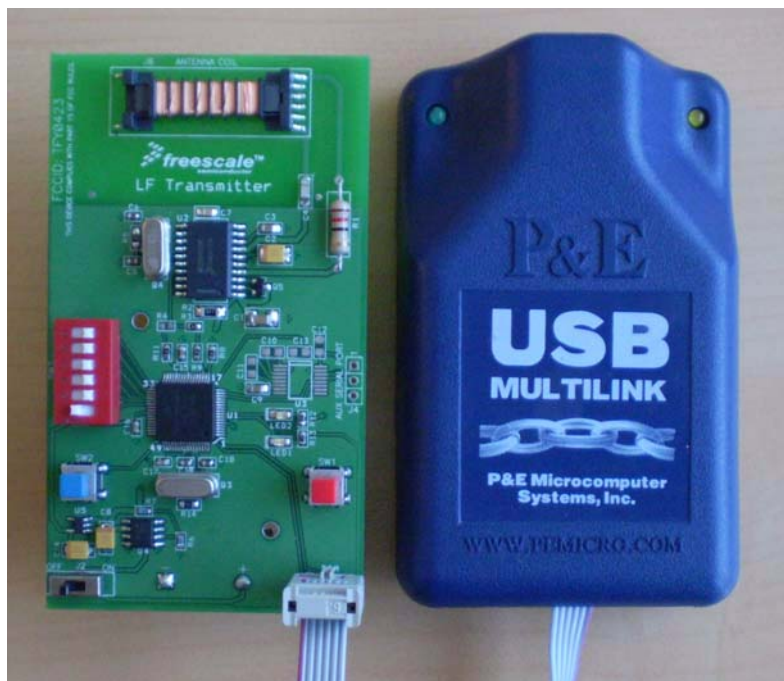
Figure 1-5. MPXY8300 and LF125kHz Connected to the USB Multilink
