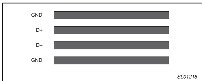
Figure 12. PCB layout for D+ and D-
