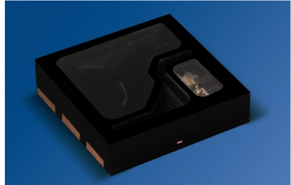
Figure 1: Photo of the SFH 7740. Contact pads are on the bottom side of the package
