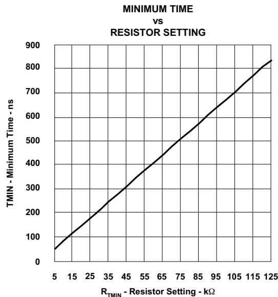
Figure 9. Minimum Time TMIN Over Setting Resistor R_{TMIN}
