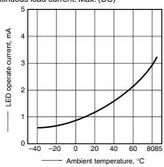
LED turn off current vs. ambient temperature characteristics
