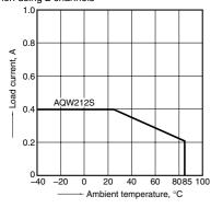
1.-(2) Load current vs. ambient temperature characteristics
