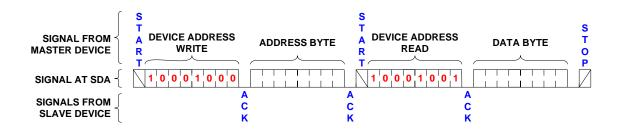
FIGURE 13. BYTE ADDRESS READ SEQUENCE
