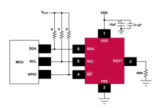
FIGURE 1. ISL29023 TYPICAL APPLICATION DIAGRAM
