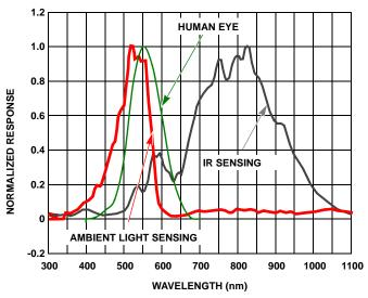
FIGURE 2. NORMALIZED SPECTRAL RESPONSE FOR AMBIENT LIGHT SENSING AND IR SENSING
