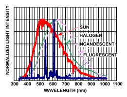
FIGURE 3. NORMALIZED SPECTRAL RESPONSE OF LIGHT SOURCES
