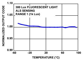
FIGURE 8. OUTPUT CODE vs TEMPERATURE
