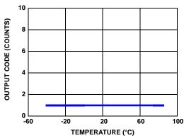
FIGURE 7. OUTPUT CODE FOR 0 LUX vs TEMPERATURE
