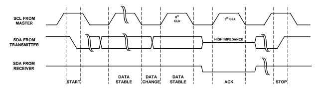
FIGURE 12. START, DATA STABLE, ACKNOWLEDGE, AND STOP CONDITION
