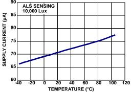
FIGURE 9. SUPPLY CURRENT vs TEMPERATURE IN ALS SENSING
